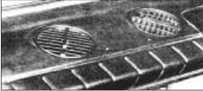
Left: the upper vents for the heating system can be swivelled to direct the air towards the occupants's faces
