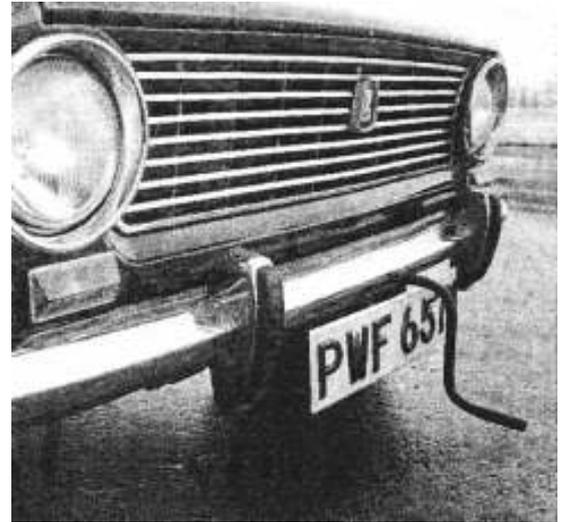
Above left: Access around the single overhead camshaft engine is very good, especially around the oil filter and fuel pump. Above right: A rare sight - the starting handle on the Lada 1200, which makes engine servicing work so easy
