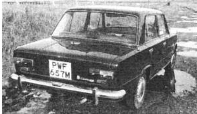
There are towing eyes built in beneath the rear bumper, which has deep overriders. The boot is key lock only
